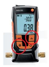
Next, press the " $\Delta$ " multiple times until a reading of at least 100 microns is reached before holding the "\*" and " $\Delta$ " buttons simultaneously again. The 552 now assumes that the vacuum pump pulls down to 100 microns. This way, if a vacuum pump capable of even lower pressures is used, the 552 will be able to show this.
