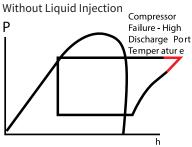
Liquid Injection protects compressor from failure by preventing too high discharge temperature. Liquid Injection helps provide wide range operating envelope.
